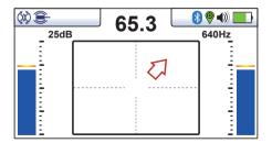
6. If the bar graph is not steady it will most likely be because the sonde is not within range. In this case hold the locator at approximately 45 degrees to the ground and rotate the locator around a full 360 degrees around you. Note the direction of strongest signal and walk towards it until the bar graph shows a steady signal. Now revert to step five above.
