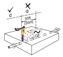
Also note that the signal will radiate out to the side of the transmitter as well as below. For this reason, it is recommended that when applying a signal using the induction method, a distance of at least 20m is kept from the transmitter when pinpointing or taking depth readings. Locating closer than 20m is possible but the operator should be aware that the signal directly received from the transmitter may be strong enough to influence the results.
