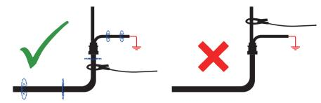
When clamping around a cable make sure the clamp is placed below the grounding point as shown below.
