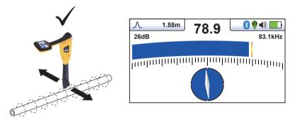
Hold the locator vertically and rotate it on its axis until the compass indicates Forward/Back as above.
