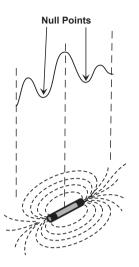
Due to this construction, the sonde gives a different "Peak" pattern note that there are three distinct peaks – a small peak – a large peak – a small peak with two "Nulls" between the peaks. The sonde is located under the center of the "large peak".
